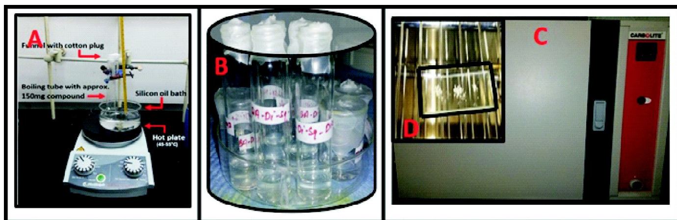
Fig. 3. Different crystallization techniques. (A) Sublimation, (B) Slow evaporation, (C) Melt crystallization apparatus, (D) Melt crystallization inside the chamber.
